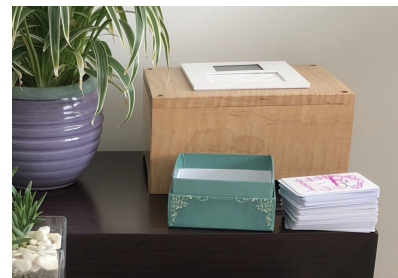
Figure 1: This FamilySong box is located in a grandparent house. A second box is located in the house of their children/grandchildren. Their Near-Field Communication (NFC) cards, are stacked next to the box and are recognized by an NFC reader on top of the box. Cards are associated to song through a web application. Once a card has been programmed with a song, placing or swiping the card over the box adds its song to the family's music queue, to play simultaneously on both houses. Additionally, participants decorate their cards to aid recognition and to personalize them.
