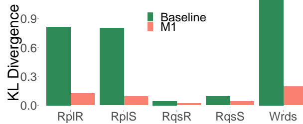
Figure 3.17: KL-divergence values for the baseline M0 and M1 models across the five parameters of x : lower values are better. The modeling conditions are experiment with k = 2 . This figure shows that M1 greatly improves a weakness of model M0 in poorly representing RplR (number of replies received), RplS (number of replies sent), and Wrds (number of words formed).
